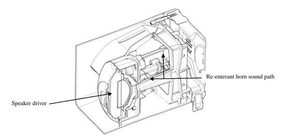
Fig 5: Electronic Horn and Siren utilizes speaker driver and reentrant horn
