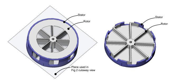
Fig 1: Rotor and stator in a typical electromechanical siren
