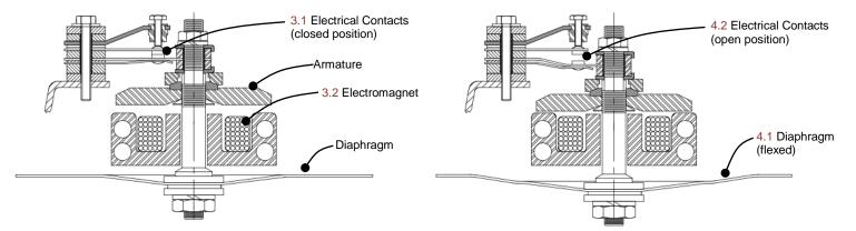
Fig 3: Electromechanical horn mechanism in an unpowered state
