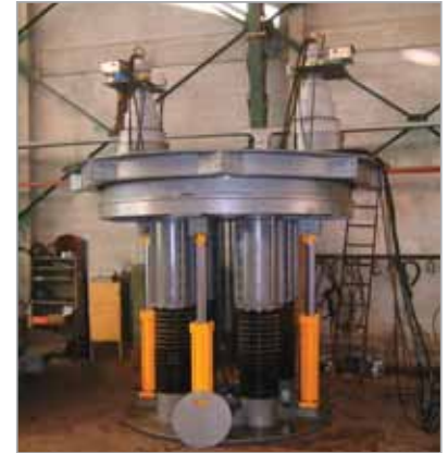
Cage Drive with Hydraulic Lift
