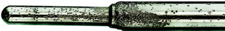
Fig. 3-31: Pitting corrosion in a Monel thermowell after usage in a chemical system
