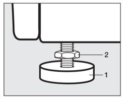
■ Turn the locking nut, **2**, counter-clockwise with the enclosed combination wrench. Unscrew each of the four feet as much as necessary by turning both the foot, **1**, and the locking nut, **2**, to the left.
