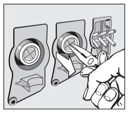
■ Using needle nose pliers, remove the plastic filter by pulling on the bar (see illustration). Rinse under running water and return. Replace the filter and seal, then reconnect the hose.
