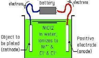
Imagine that we have an object that is made of copper or steel, and that it has been properly cleaned, and that we now want to plate it with nickel. A wire is attached to the object, and the other end of the wire is attached to the negative pole of a battery (the wire is blue in this picture). To the positive pole of the battery we connect the red wire; the other end of the red wire we connect to a rod made of nickel.
