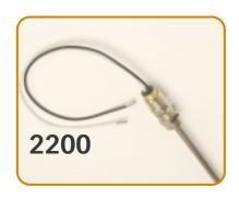
An Alloy 825 stainless steel-sheathed MI cable with solid nickel conductors and magnesium oxide insulation, System 2200 cables provide fire protection with exposure temperatures to 2200°F (1200°C)
