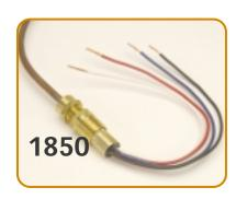
A flexible, copper-sheathed MI cable with solid copper conductors, System 1850 cables operate continuously to 482°F (250°C) with exposure temperatures to 1850°F (1010°C)
