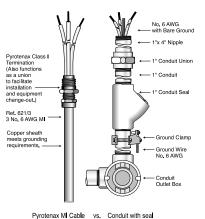
Pre-terminated MI circuits used in hazardous area gas-path-blocked applications eliminate the time and materials used in conventional conduit and wiring methods while a smaller overall profile permits more cable runs in less space.
