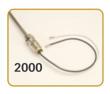
An Alloy 825 stainless steel-sheathed MI cable with nickel-clad copper conductors and magnesium oxide insulation, System 2000 cables provide fire protection with exposure temperatures to 1950°F (1065°C)
