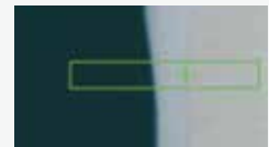
Edges are detected reliably even when the contrast between the background and subject is low.
