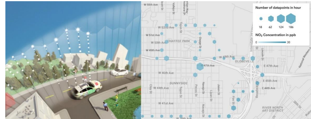
Example of Mapping Air Pollution Levels for NO 2 by Sensors Instrumented by Aclima Onto Google Cars
