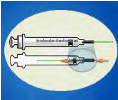
Syringe with retractable needle.
