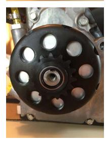
Properly spaced clutch. The clutch will be clamped tight on the crankshaft to minimize fretting of keyway and potential damage to the integral keys.
