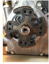
Install the spring/shoe retaining washer.
