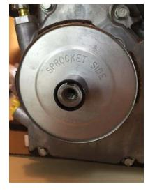
Install the drum/sprocket assembly.
