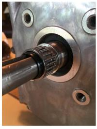
Install the drum/sprocket assembly. The sprocket will slide over the needle bearing easier if you rotate the drum while installing.
