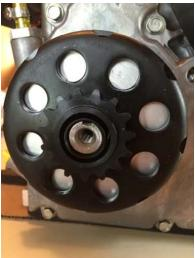
Lubricate the needle bearing with a high temperature bearing grease and install.
