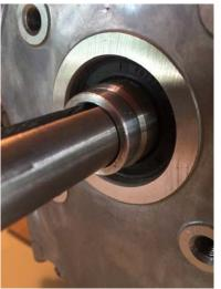
Install the  $\frac{3}{4}$ " x 1 1/16" OD x .04" thick steel washer against the crankshaft spacer.
