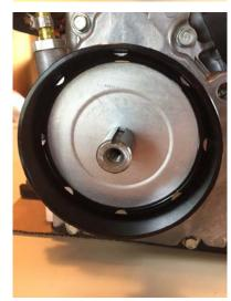
Install the spring/shoe retaining washer.
