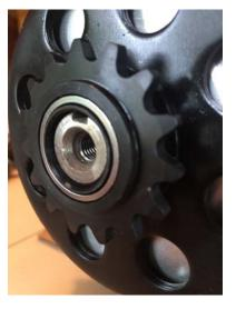
Install the bolt, lock washer, and mounting washer. Properly torque to the engine manufacturer specifications.
