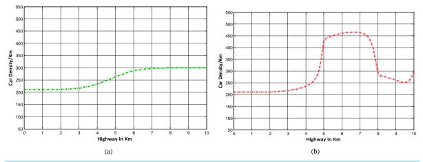
**Figure 6.** (a) Density profile simulation for 6 minute without any inflow or outflow; (b) Density profile simulation for 6 minutes with an inflow at  $5^{\text{th}}$  km position and outflow at  $8^{\text{th}}$  km position.
