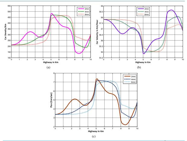
Figure 5. (a) Density profile and (b) Velocity profile and (c) Flux profile in 10 km highway with inflow at  $5^{th}$  km position and outflow at  $8^{th}$  km position.
