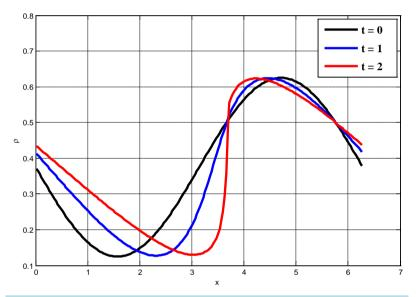
Figure 8. Numerical solutions using Godunov method in different time steps.
