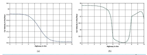
Figure 7. (a) Corresponding velocity profile without any inflow or outflow; (b) Velocity profile with an inflow at  $5^{th}$  km position and outflow at  $8^{th}$  km position.
