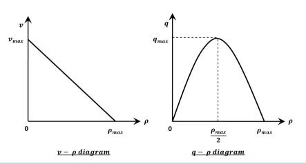
**Figure 1.** The fundamental  $v - \rho$  diagram and  $q - \rho$  diagram according to Greenshields.
