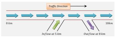
Figure 3. Layout of a 10 km highway with an inflow source term at 5<sup>th</sup> km and outflow sink term at 8<sup>th</sup> km position.
