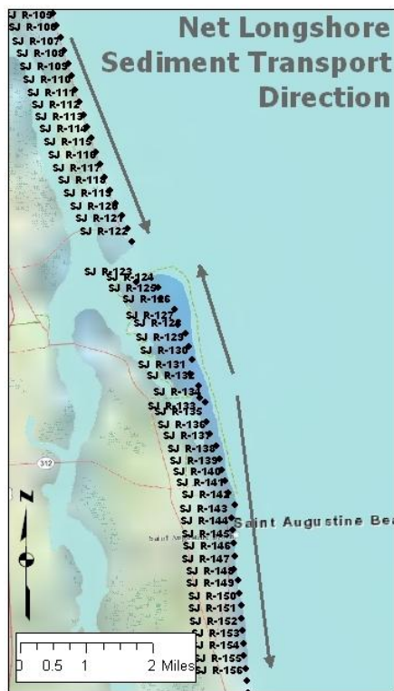
Figure 2. General net longshore sediment transport directions in the vicinity of the inlet.
