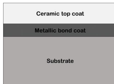
Figure 1. A schematic of a typical thermal barrier coating system showing all the layers which are from the top-bottom: Ceramic top coat, Metallic bond coat and Substrate.
