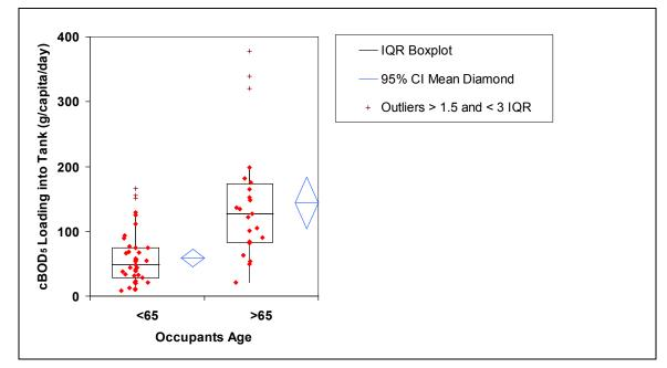
Figure 4-30. Mass Loading Rates of Raw Wastewater into the Septic Tank for cBOD<sub>5</sub> by Age of Occupant.
