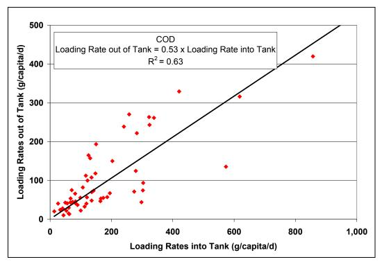
Figure 4-33. Correlation between COD Mass Loading Rates of Raw Wastewater into the Septic Tank and of STE out of the Septic Tank.
