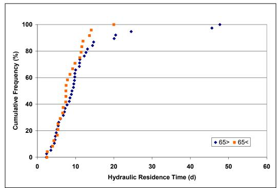
Figure 4-1. Hydraulic Residence Time in the Septic Tank by Age of Occupant.
