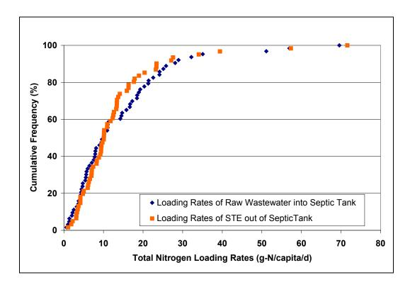
Figure 4-26. Mass Loading Rates for Total Nitrogen.
