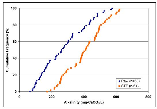
Figure 3-8. Alkalinity in Raw Wastewater and STE.
