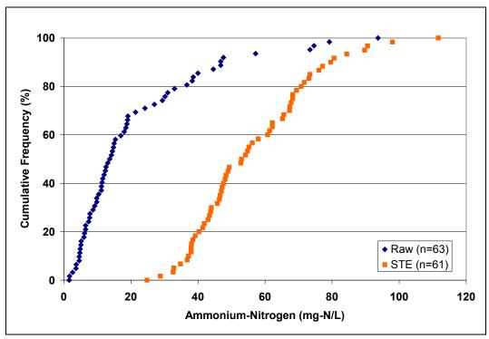
Figure 3-17. Ammonium-nitrogen in Raw Wastewater and STE.
