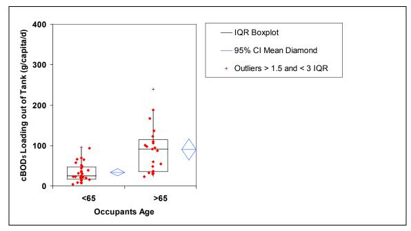
Figure 4-31. Mass Loading Rates of STE out of the Septic Tank for cBOD<sub>5</sub> by Age of Occupant.
