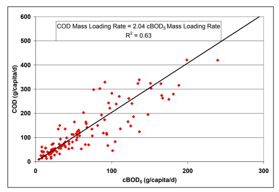
Figure 4-36. Correlation between  $cBOD_5$  and COD Mass Loading Rates of Raw Wastewater into the Septic Tank combined with STE out of the Septic Tank.
