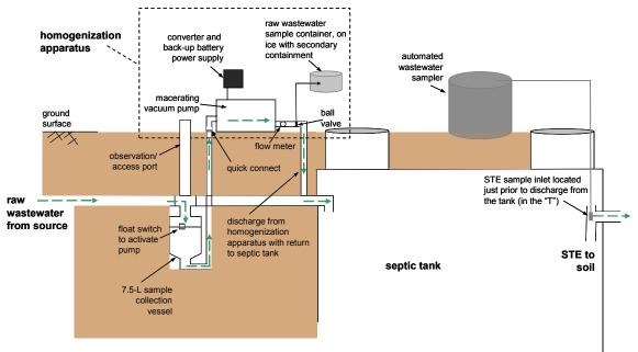
Figure 2-1. Illustration of Raw Wastewater and STE Collection Approach (not to scale).
