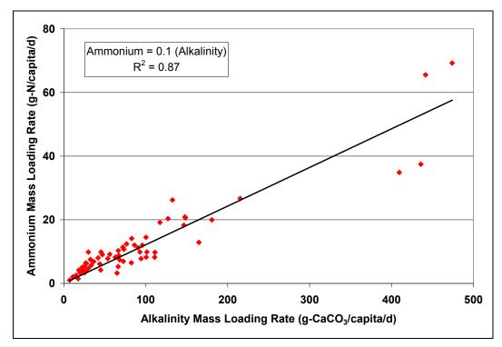
Figure 4-37. Correlation between Alkalinity and Ammonium-nitrogen Mass Loading Rates of Raw Wastewater into the Septic Tank combined with STE out of the Septic Tank.
