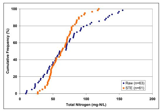
Figure 3-15. Total Nitrogen in Raw Wastewater and STE.
