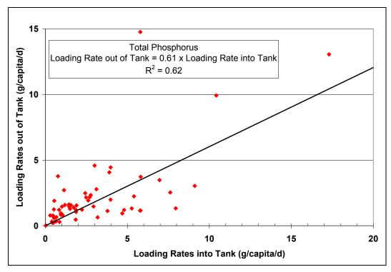
Figure 4-35. Correlation between Total Phosphorus Mass Loading Rates of Raw Wastewater into the Septic Tank and of STE out of the Septic Tank.
