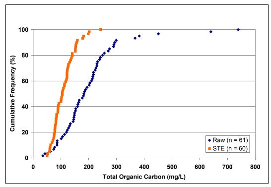
Figure 3-13. TOC in Raw Wastewater and STE.
