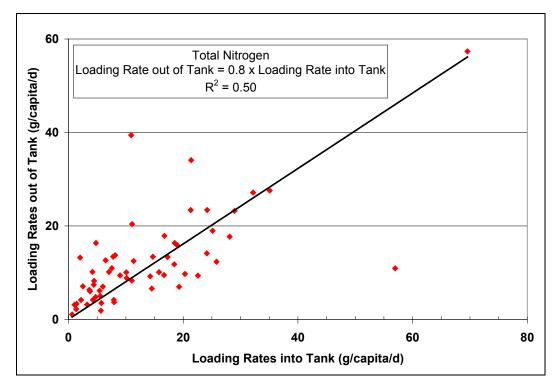
Figure 4-34. Correlation between Total Nitrogen Mass Loading Rates of Raw Wastewater into the Septic Tank and of STE out of the Septic Tank.
