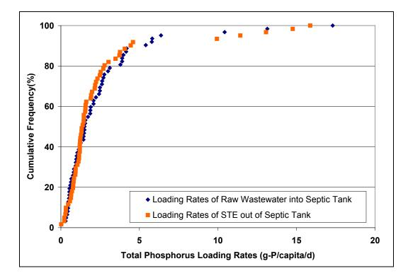
Figure 4-27. Mass Loading Rates for Total Phosphorus.
