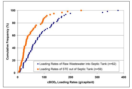
tank (68 and 32 g/capita/d respectively) suggested cBOD<sub>5</sub> mass removal of approximately 50% in the septic tank. Similar mass loading rate trends were found for COD (Figure 4-25).
