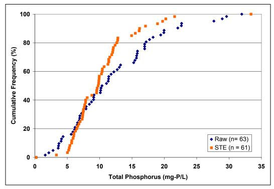
Figure 3-19. Total Phosphorus in Raw Wastewater and STE.
