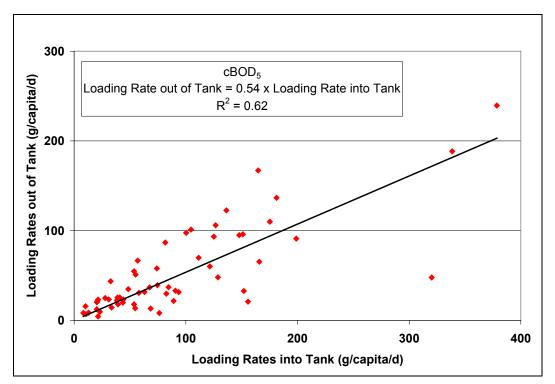
Figure 4-32. Correlation between cBOD<sub>5</sub> Mass Loading Rates of Raw Wastewater into the Septic Tank and of STE out of the Septic Tank.
