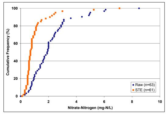
Figure 3-18. Nitrate-nitrogen in Raw Wastewater and STE.
