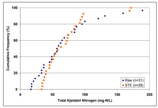
Figure 3-16. TKN in Raw Wastewater and STE.
