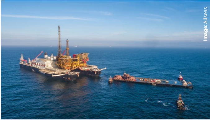
Moving the Iron Lady into the Pioneering Spirit 's bow slot
