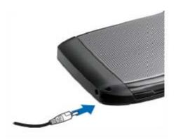
3. When the battery is fully charged, disconnect the charger from the device, then from the wall outlet. Your battery has been precharged at the factory, but the charging levels may vary. To reach the full operation time, charge the battery until it has been fully charged according to the battery level indicator.
