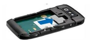
4. Insert the battery. Align the contacts of the battery with the corresponding connectors on the battery compartment and insert in the direction of the arrow.
