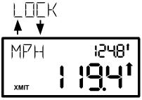
124.8 MPH when the trigger was pressed to lock its speed. After the lock, the target has slowed to 119.4 MPH.
