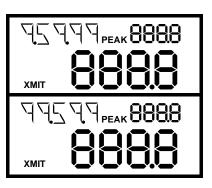
**Cosine Angle:** This setting is used to automatically correct speed readings for angle errors. It can be set in one degree increments in the range from 0 through 45 degrees. The default setting is 0 degrees. Refer to the Angle Errors section for more details.
