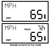
When Peak mode is ON, the PEAK icon appears on the display and the highest speed attained displays in the upper right window. The live vehicle speed displays in the main window.
