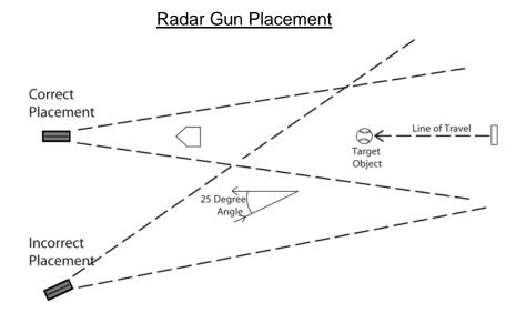
At slight angles the error is very small; however at larger angles, the error becomes substantial as the table below shows.
