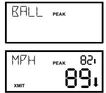
\* When the gun **IS** transmitting, the XMIT icon is on and the unit of measure displays in the message window.
