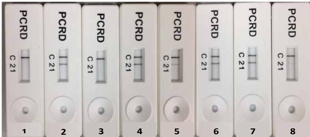
Figure 1. RPA-LFA test results show negatives as one control band (Nos. 1 and 3), positives as two bands (Nos. 2, 4, 6, 7), and faint positives indicating very low levels of DNA present (Nos. 5 and 8).
