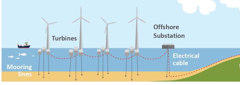
3. A transmission cable transmits the power from the floating substation to the shore, where it is connected to the onshore electric system.
