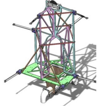
Design concepts for a cable driven large format AM system for the production of construction scale structures **Materials Development:** Development of extrudable thixotropic concrete materials which exhibit sufficient structural performance and processing characteristics which are beneficial for system performance (i.e. low slump, pumpable, quick set time, high early strength)
