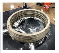
Concepts and hardware have been developed to evaluate the efficacy of low cost AM for the construction of infrastructure scale structures
