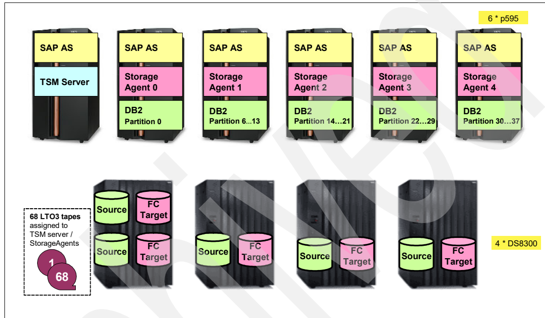
Figure 6-6 Tivoli Storage Manager and Data Protection design
