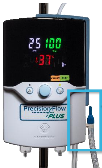
Electronic Components; Input Gas Controls
