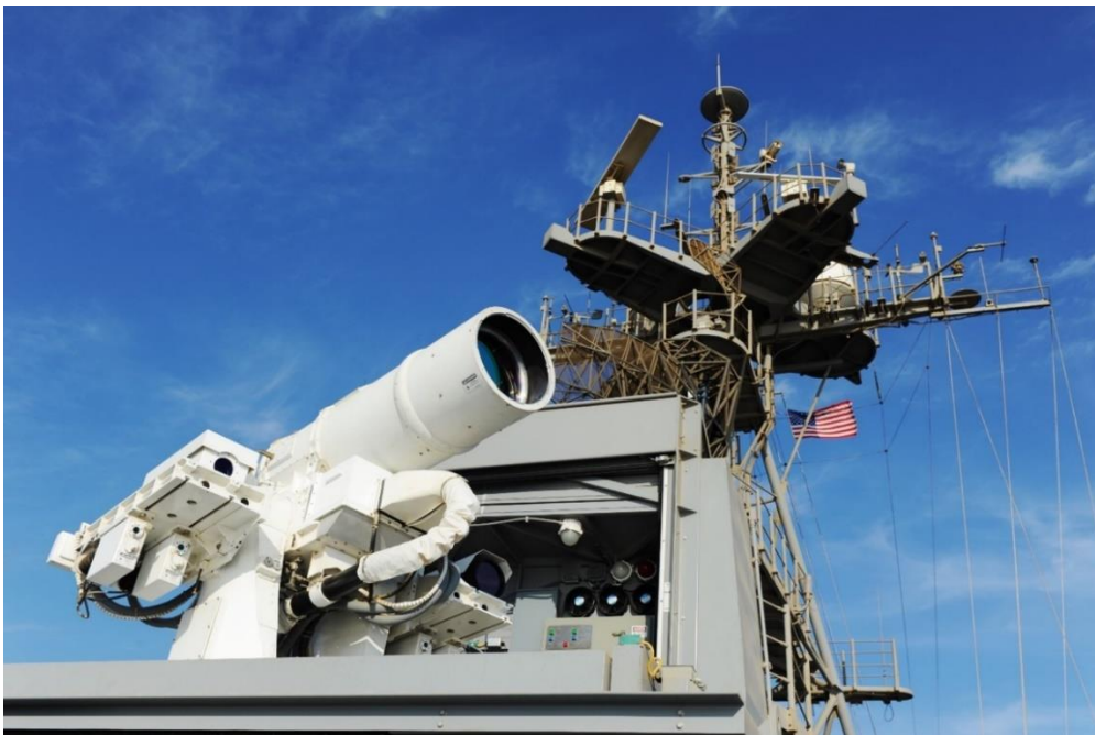
The US Navy's AN/SEQ3 laser system.
