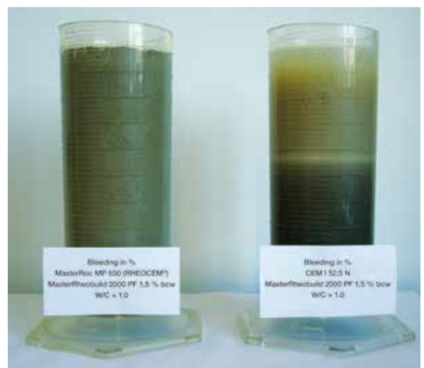
Stable (left) vs. unstable (right) grout
