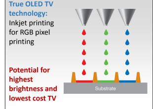
Most efficient use of RGB materials, no color filter or shadow mask
