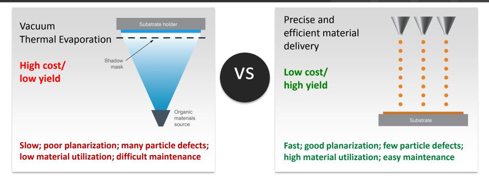
Many solutions were tried, but Kateeva's inkjet printing was the solution that enabled costeffective encapsulation for mobile flexible OLED displays in mass production
