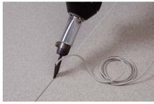
Weld rod seam
