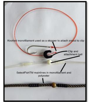
Figure 6: Components of SelectFish system
