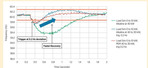
Figure 35. Use of electrolyser for fast frequency response
