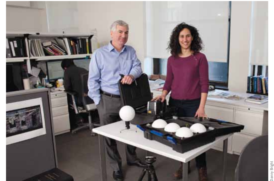
Tom Duffy and Francesca Brando, a senior engineer, pack up the 3DS 120 laser scanner. The white globes are reference spheres, artificial targets used to register multiple scans so they can be combined into a complete point cloud.
