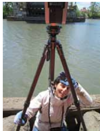
To hold the 3DS 120 laser scanner steady on a windy day in the field, Viviana Vumbaca finds one of the scanner's few blind spots.
