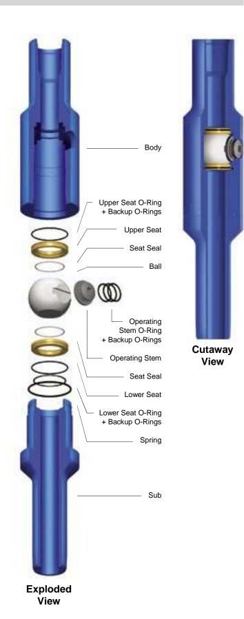
Packard International's safety valves are designed for even the harshest drilling conditions; however, it is suggested that parts most subject to wear and tear be replaced regularly.
