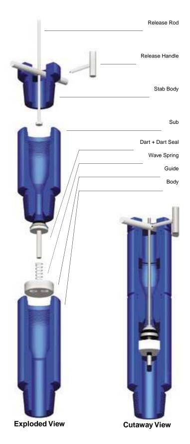
The Packard International IBOP is designed for the harshest drilling environments, however it is suggested the parts most subject to wear be replaced at regular intervals.
