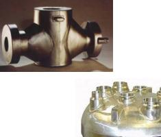
3. Hot Isostatic Pressing Apply High Pressure (>15,000psi), Temperature (>2000F)
