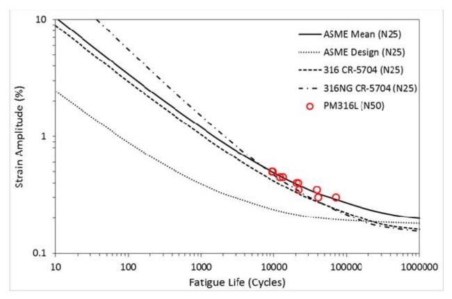
Measured 316LSS LCF data compared with ASME and NUREG- 5704 data.
