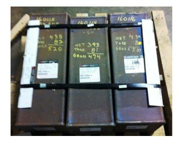
3 Test SA508 Class 1, Grade 3 Test Blocks
