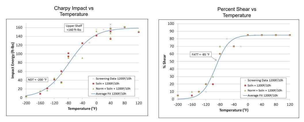
Solution Annealed at 2050F/10hrs, quenched, normalized 1650F and tempered at 1200F/10 hrs
