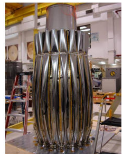
Figure 47: Stowed TacSat-4 UHF Antenna retained by a belt split spool system (Image credit: Naval Research Laboratory)
