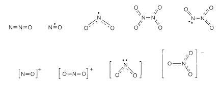
Fig. 2. Structures of some oxides, oxocations and oxoanions of nitrogen.
