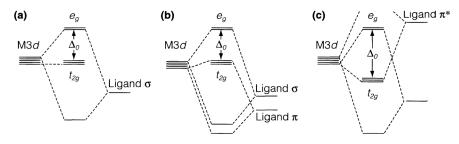
Fig. 2. Partial MO diagram showing an octahedral complex with (a)  $\sigma$ -donor only, (b)  $\pi$ -donor, and (c)  $\pi$ -acceptor ligands.
