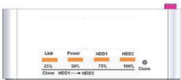
**NOTE:** If cloning operation fails, LED on HDD2 flares in red, leaving the other LEDs off.
