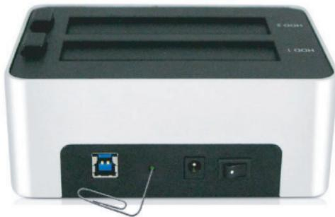
**STEP 4:** LEDs will flash sequentially, indicating the erasing is in progress. Each red LED refers to 25% of erasing completion.
