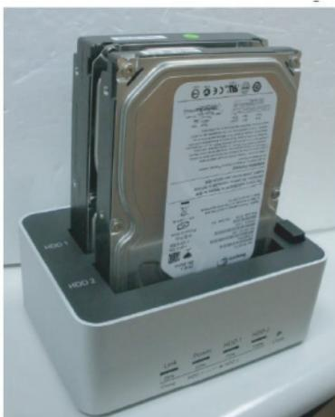
**STEP 2:** Make sure power is turned on and USB cable is NOT connected.
