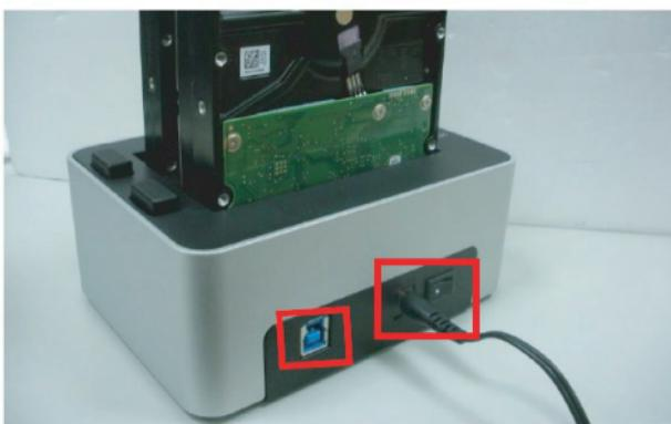
**STEP 3:** Pin and hold the erase button for at least 5 seconds, then erasing operation will start by indicating all 4 LEDs in red.
