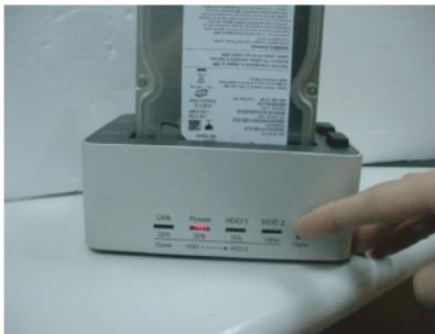
**STEP 4:** LEDs will then proceed to flash sequentially indicating the cloning is in progress. Each orange LED refers to every 25% of cloning completion. It is only when every 25% of HDD1 is cloned to HDD2 that such LED will remain constantly on, leaving the other LED(s) in running stage. When cloning operation is fully completed, all LEDs will flash regularly in orange.
