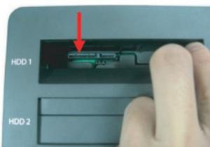
**Step 2:** Install the hard drives HDD/SSD 2.5" and/or 3.5" in the docking station, with the SATA connector and the port aligned.
