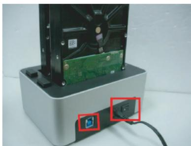
**STEP 3:** Press & hold the cloning button for at least 5 seconds, then cloning operation will start, indicating all 4 LEDs in orange.
