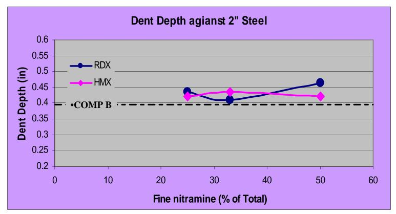
PAX 40 & 41 exhibit larger dent depths than COMP B consistent with higher detonation pressures.
