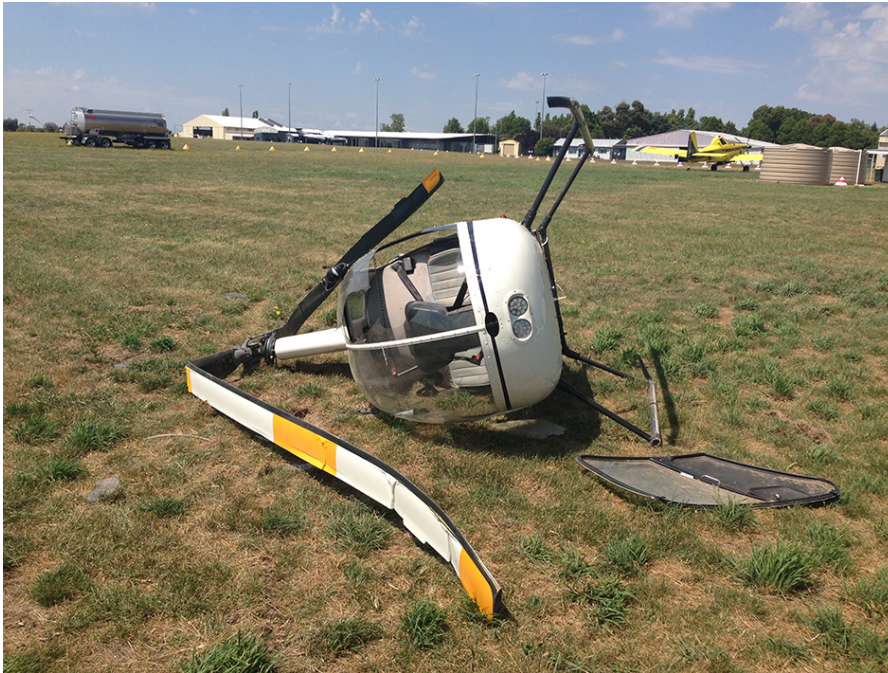
Figure 2: Detached right door and damaged rotor blades
