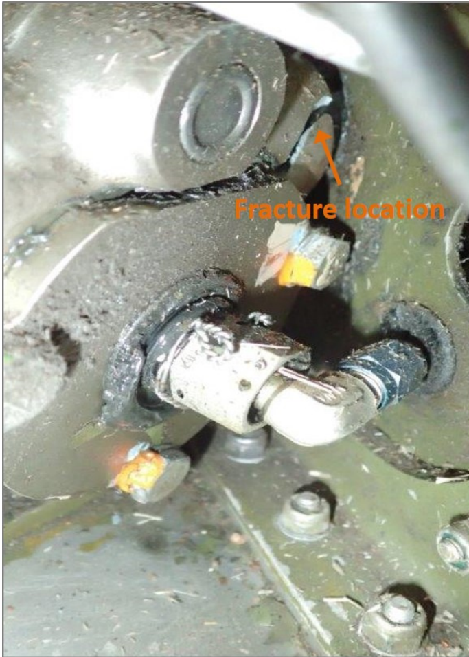
Figure 2: JGA left main landing gear actuator showing the fractured housing
