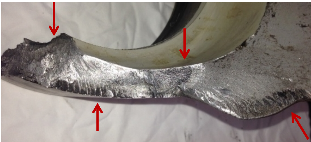
Figure 3: Secondary, circumferential crack showing, from left to right, the damaged origin area, ratchet marks/burnishing, beach marks and ultimate failure by overload
