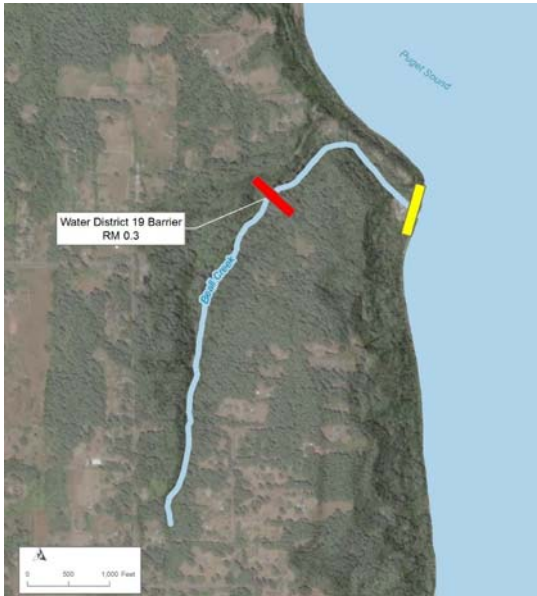
4252 Figure 2. Beall Creek with a partial fish passage barrier at river mile 0.02 (yellow) and a complete fish passage 4253 barrier at river mile 0.30 (red). Both locations are associated with Water District 19. This project is focused on flow 4254 improvements at river mile 0.30. 4255 4256
