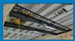
6 Ton X 40' Approx. Span Cleveland Tramrail Double Girder Top Running Overhead Bridge Crane
