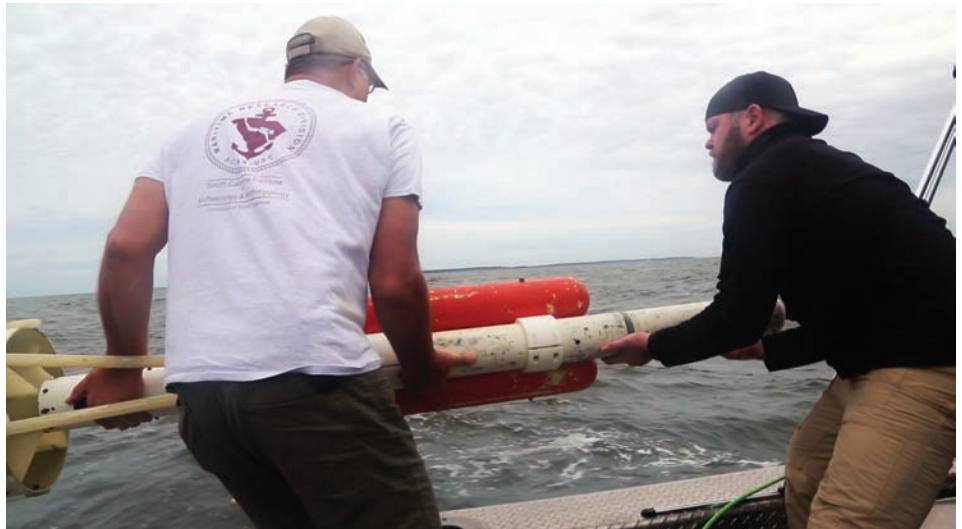
Figure 2: Jim Spirek and Ryan Bradley heaving the magnetometer sensor overboard the survey vessel. (SCIAA photo)
