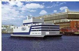
Key facts: An FNPP is basically a mobile, low-capacity reactor unit operable in remote areas isolated from the main power distribution system, or in places hard to access by land. They are designed to maintain both uninterruptible power and plentiful desalinated water supply in remote areas.
