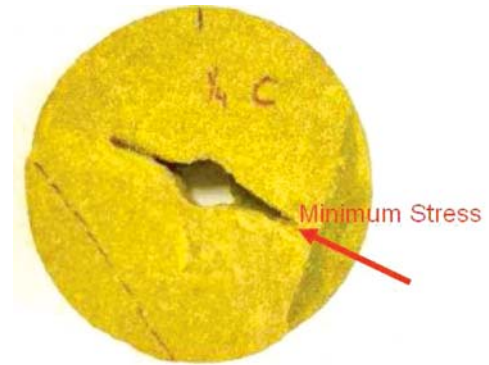
Fig 13: SPE 98315 – Failure Shape Courtesy of J.C. Heiland & M.E. Flor – SPE 98315
