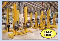
(3) Sets of SEFAC Model M150BF2800 Mobile Lifting Jacks
