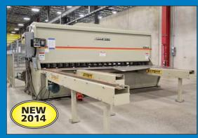
1/2" x 14' AccurShear Model 650014 CNC Hydraulic Shear
