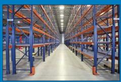
(78) Sections of 9' W x 42" Deep x 26' H Tear-Drop Adjustable Beam Pallet Rack
