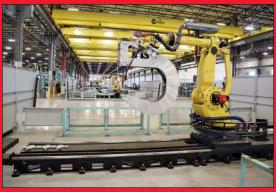
\*\*(4) Genesis / Fanuc Track-Mounted Single-Robot Spot Welding Cells
