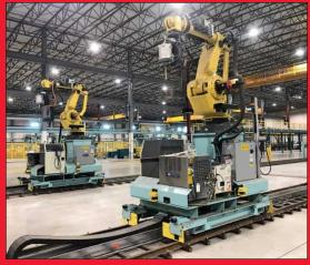
(2) Genesis / Fanuc Track-Traveling Single-Robot Spot Welding Systems
