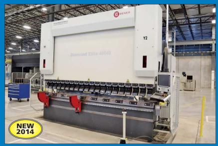
440 Ton X 159" Dener Model DE400-40-AC-ZL-2M Multi-Axis CNC Press Brake
