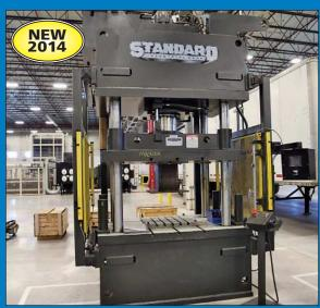
200 Ton Standard Industrial Model AP200-48-48 Four-Post Vertical Hydraulic Press
