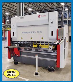
(2) 88 Ton X 102" Dener Model DE80-26-AC-ZL-2M Multi-Axis CNC **Press Brakes**
