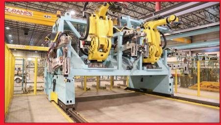
Genesis / Fanuc Track-Traveling Two-Robot Spot Welding System
