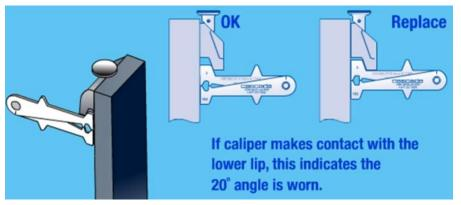
Calibers can be used to inspect the fork hooks for signs of wear or bending
