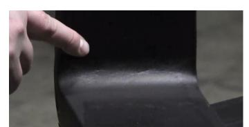
Blades with surface cracks should not be used until they are approved or repaired by a competent person.
