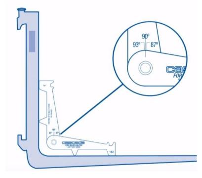
Fork Angle: Forks are made with a 90 degree angle. Forks with a different angle may need to be corrected or replaced. A special caliper to measure the angle of the forks is used. The caliper is simply aligned to that it touches both the shank and the blade by the heel. The caliper is marked to show the allowable deviation of 3 degrees either way of a perfect 90 degrees.
