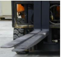
**Straightness of Blade and Shank**: The straightness of the upper face of the blade and the front face of the shank should be checked. If the deviation from straightness exceeds 0.5% of the length of the blade and/or the height of the shank, respectively, the fork should be taken out of service and not returned to service until it has been properly repaired.
