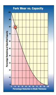
The graph on the left shows how the specified capacity of a forklift blade decreases as the blade thickness decreases. Blade thickness decreases as the blades are worn down by rubbing on the floor and on pallets. The wear happens slowly and the blade may be fine for years but the blade will eventually start to wear down and get thinner.
