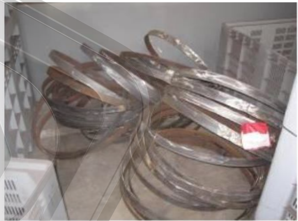
Splicing backing rings: 860x6mm
