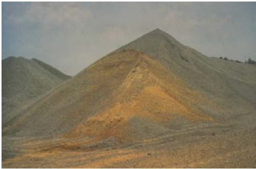
Photo 4. Stockpile contaminated with underlying materials.
