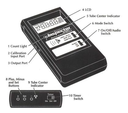
The Inspector Alert counts ionizing events and displays the results on the liquid crystal display (LCD) (4). You control which unit of measurement is shown by using the mode switch.
