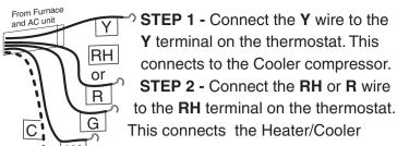
This connects the Heater/Cooler Power. STEP 3 - Connect the W wire to the W terminal on the
