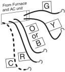
**STEP 1 -** Connect the **G** wire to the **G** terminal on the thermostat.
