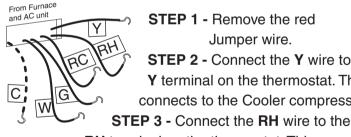
STEP 1 - Remove the red Jumper wire.
