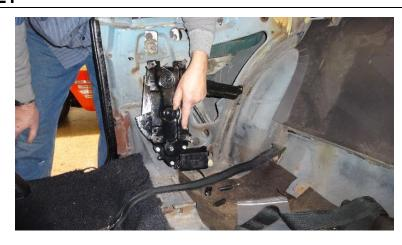
Here are the bolt locations for the 2 regulators. The RED Xs were the locations of the factor regulator bolts and the GREEN are factory holes that you will now be using and the YELLOW are the holes you drilled at the beginning of the Quarter Prep.
