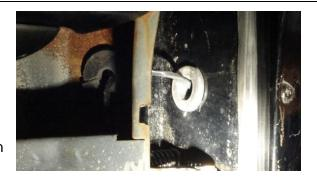
The power window regulator does not use the same holes as the manual regulator. This picture shows the approximate orientation of the new regulator when it is installed in the door.
