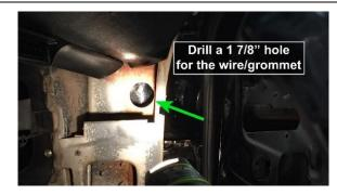
Locate the middle dimple on the door and drill a 1 1/8" hole for the wiring conduit and grommet.
