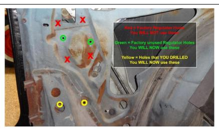
in and rotate the regulator to a 90-120 degree angle from the mounting plate. This will aid you when you place it in the quarter and when putting the wheel from the regulator into the window channel.
