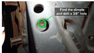
Locate the dimple to the right of the body support about the same height from the floor as the previous step and drill a 3/8" hole.
