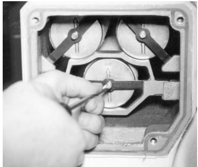
Fig. 3 - Removing the Filter Spring
