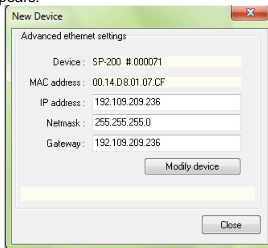
Fig. 31: “Advanced Ethernet settings” of the “New Device” window used to change the instrument IP Address.
